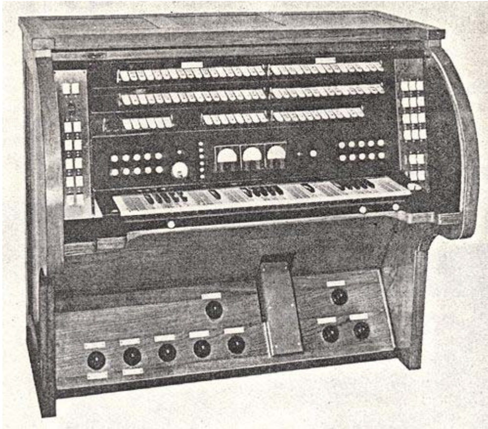
STRAND LIGHT CONSOLE DESK AT CARACAS UNIVERSITY, VENEZUALA, controlling both incandescent and fluorescent lighting.
