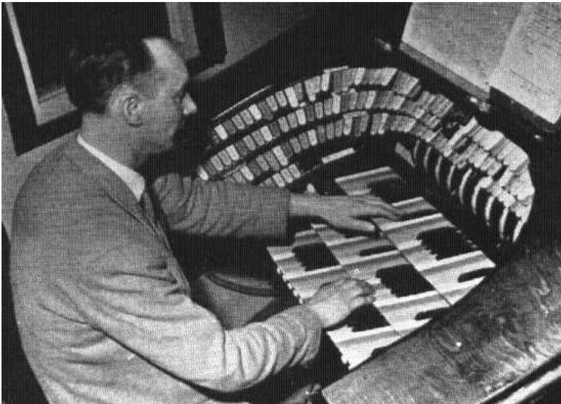
Drury Lane Theatre. Strand Light Console, 216 dimmers (Photo by courtesy "Radio Times").
