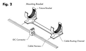
Note: One unoColor Cove power supply supports a 70-foot master cable, and each master cable supports up to thirty 12-inch fixtures or fifty 6-inch fixtures. If your installation requires more than thirty fixtures, additional connectors can be purchased from Color Kinetics. Installations larger than thirty 12-inch or fifty 6-inch fixtures will require additional power supplies.
