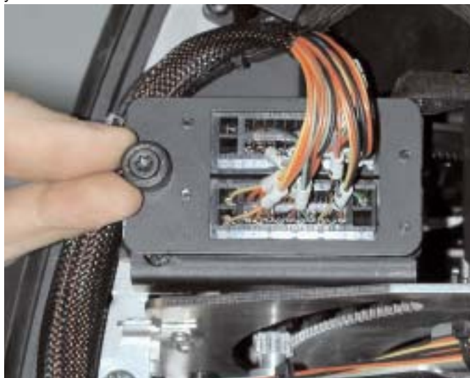
Figure W15: Disconnecting Color+Gobo+Effect Module Harness
