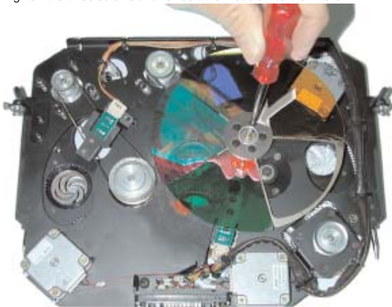
Figure W16B: Loosen Screws on Color Wheel
