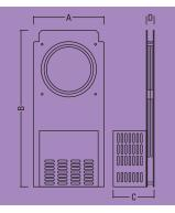
Product Code: Width (A): Height (B): Depth overall (C): Depth body only (D): Weight: Gobo size: Suitable for: Speed Range: Power Consumption: GR2D 119mm / 4.7" 263mm / 10.4" 69mm / 2.7" 13mm / 0.5" 1.1kg / 2.5lbs B Source 4 0.3 - 24rpm 0.6PU
