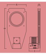
Product Code: Width (A): Height (B): Depth overall (C): Depth body only (D): Weight: Gobo size: Suitable for: Speed Range: Power: GR2FX 119mm / 4.7" 249mm / 9.8" 69mm / 2.7" 13mm / 0.5" 0.9kg / 2lbs B Source 4 Junior 0.4 - 25rpm 100 - 240VAC
