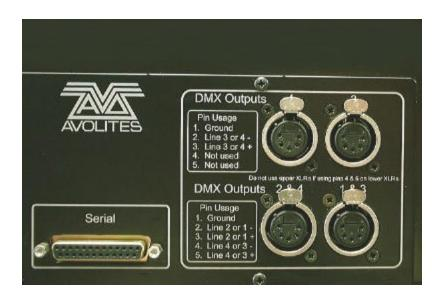
Output panel now has 4 DMX XLR connectors, as used on the Sapphire 2000.
